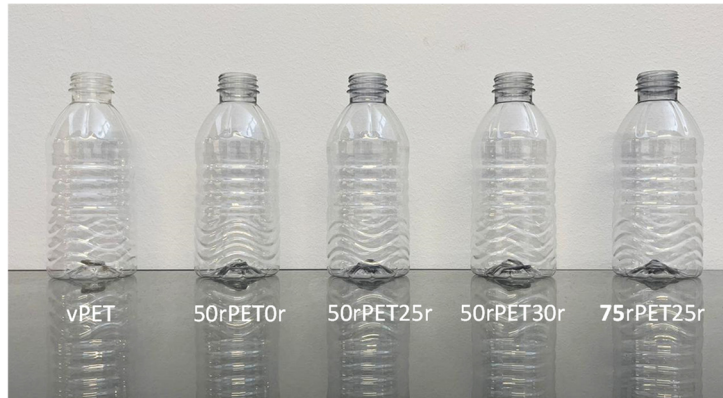
Figure 1. Image of bottles obtained with different amounts of rPET.
